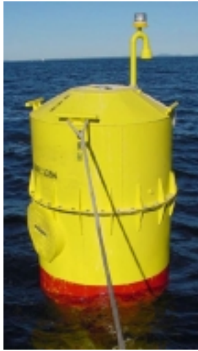
Fig. 5. Surface feed buoy platform for controlling the feeding operation, observing the fish in the cage below and telemetering the images to shore [2].
