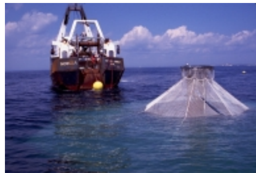
Fig. 1. Photograph of the Ocean Spar fish cage at the surface during deployment. These cages have been used to raise summer flounder, haddock and cod. The cage that was imaged during this study was submerged and was being used to raise halibut. The commercial fishing boat in the background was deploying the mooring system for the fish cage system [2, 3, 4].
