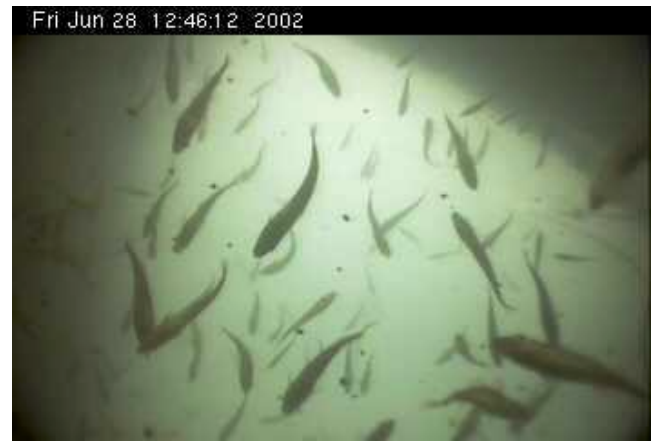
Fig. 12. Small (about 6-8") cod fish from the SeaCam in an upward looking configuration imaging the fish near and far from the camera in a coastal fish cage. The black dots between the fish are feed pellets that were thrown into the cage to simulate the release of feed by the feed buoy.
