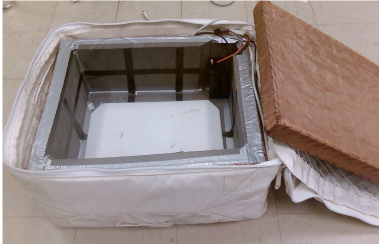
Figure 14. Single-height CTB with HF RFID Reader
