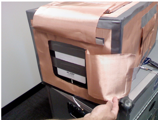
Figure 15. Antenna within CTB-proxy shielded insert
