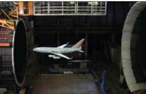
The European Active Aeroelastic Aircraft Structures project tests an adaptive aircraft design concept with a wingtip leading-edge device developed using MDO in the 7-m-diam wind tunnel at TsAGI.
