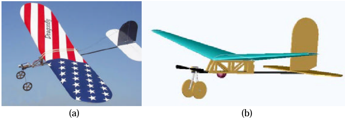
Fig. 1: (a) Baseline Dragonfly aircraft ( http://flydma.com/planes/dragonfly.html ), (b) Dragonfly “The Wing Bearer” (G. Barter, C. Johnson – Spring 2002) with modified wing for maximum endurance.
