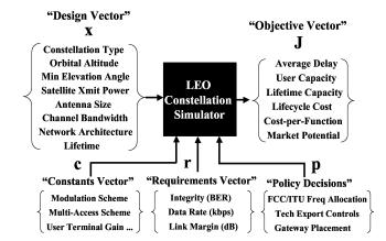
Fig. 4 Input-Output Mapping Of LEO Communication Constellation Model
