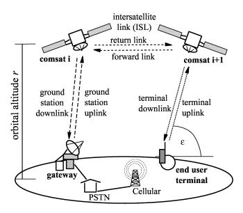
Fig. 2 LEO Communication Constellation Architecture. The end user terminal connects to a satellite comsat i+1 via the terminal up/downlink when outside of cellular coverage. Voice and data is transferred to comsat i via intersatellite link. The downlink to a ground station (gateway) provides connectivity to the Public Switched Telephone Newtork (PSTN) and wireless cellular systems.
