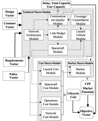
Fig. 5 LEO Communications Constellation Simulation Block Diagram
