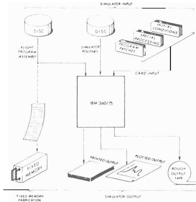
Fig. 2 Simulation system schematic
