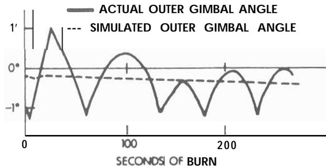
Fig. 6 Comparison of outer gimbal angles for original simulation
