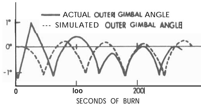
Fig. 7 Comparison of outer gimbal angles for revised simulation
