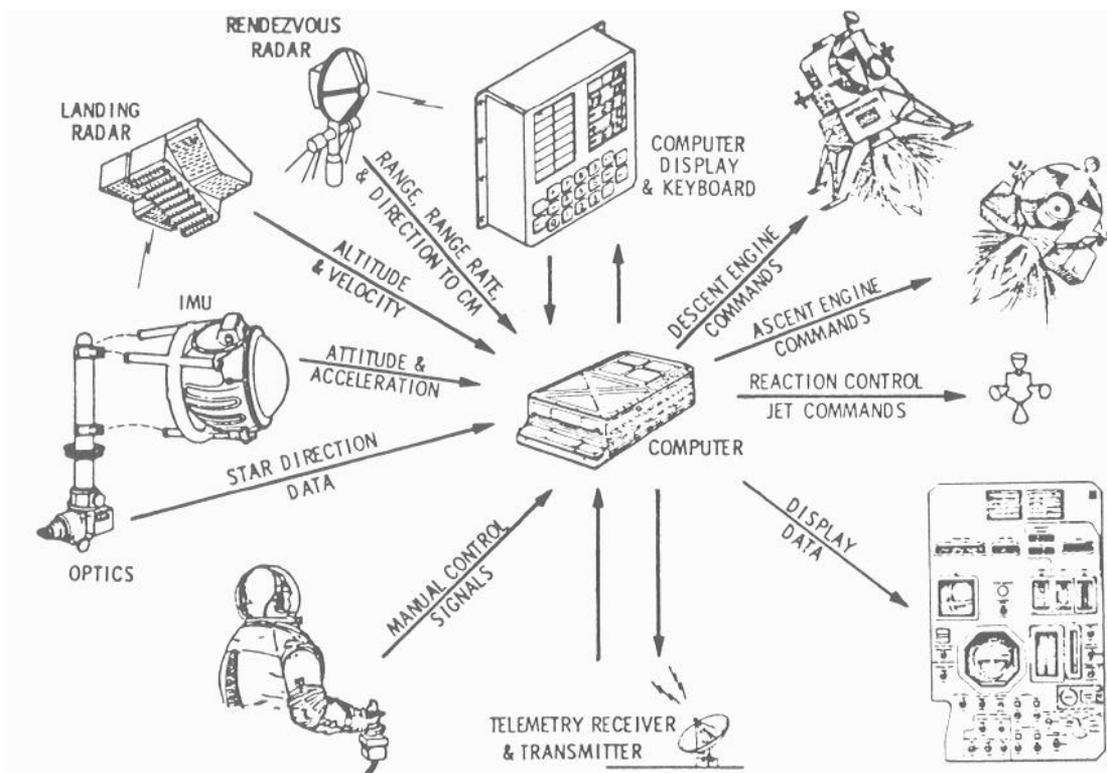
Fig. 1 The Lunar Module Computer Interfaces
