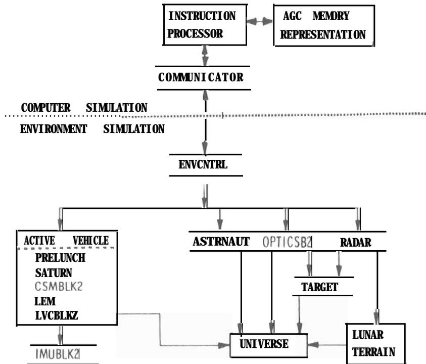
Fig. 3 Simulator routine structure
