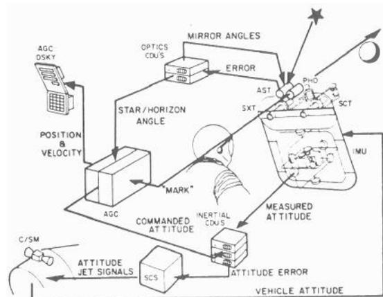
Fig. B4 Midcourse Navigation, Automatic Star-Earth Horizon Measurement
