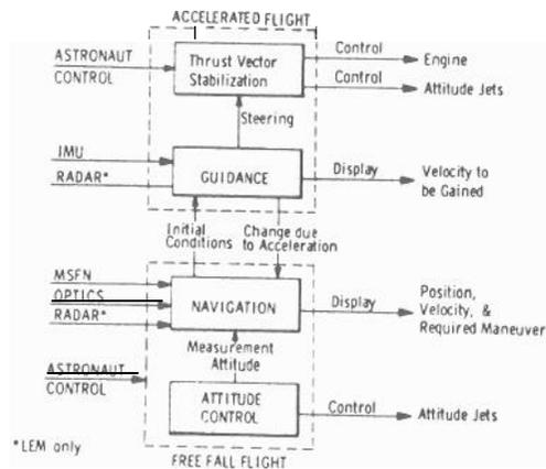
Fig. A3 G&N Function Flow
