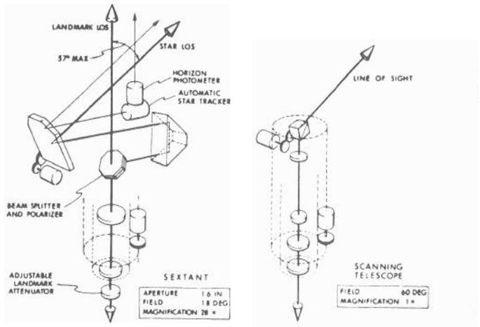
Fig. A7 Optical Schematics
