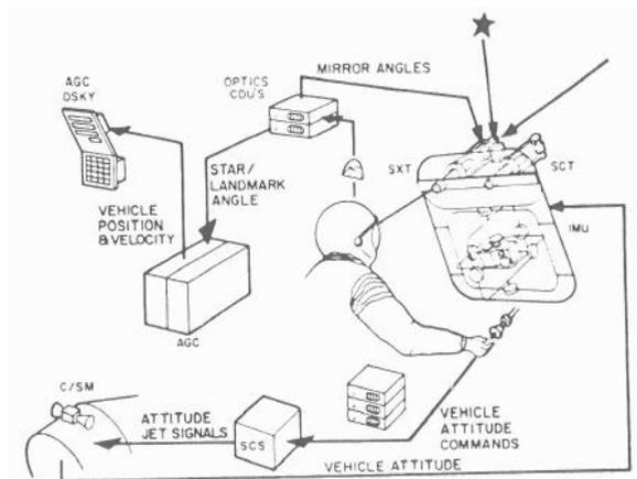
Fig. B3 Midcourse Navigation, Manual Star-Landmark Angle Measurement
