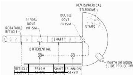
Fig. C21A SCS Simulation - Functional Schematic
