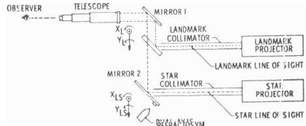
Fig. C18A Sextant Simulation - Functional Schematic
