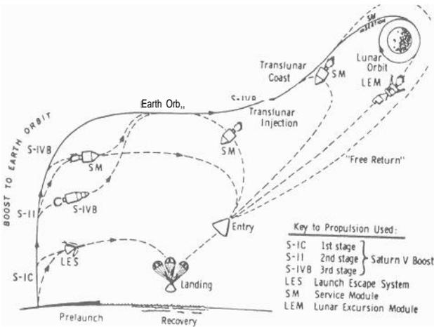
Fig. A2 Propulsion Failure Abort Paths
