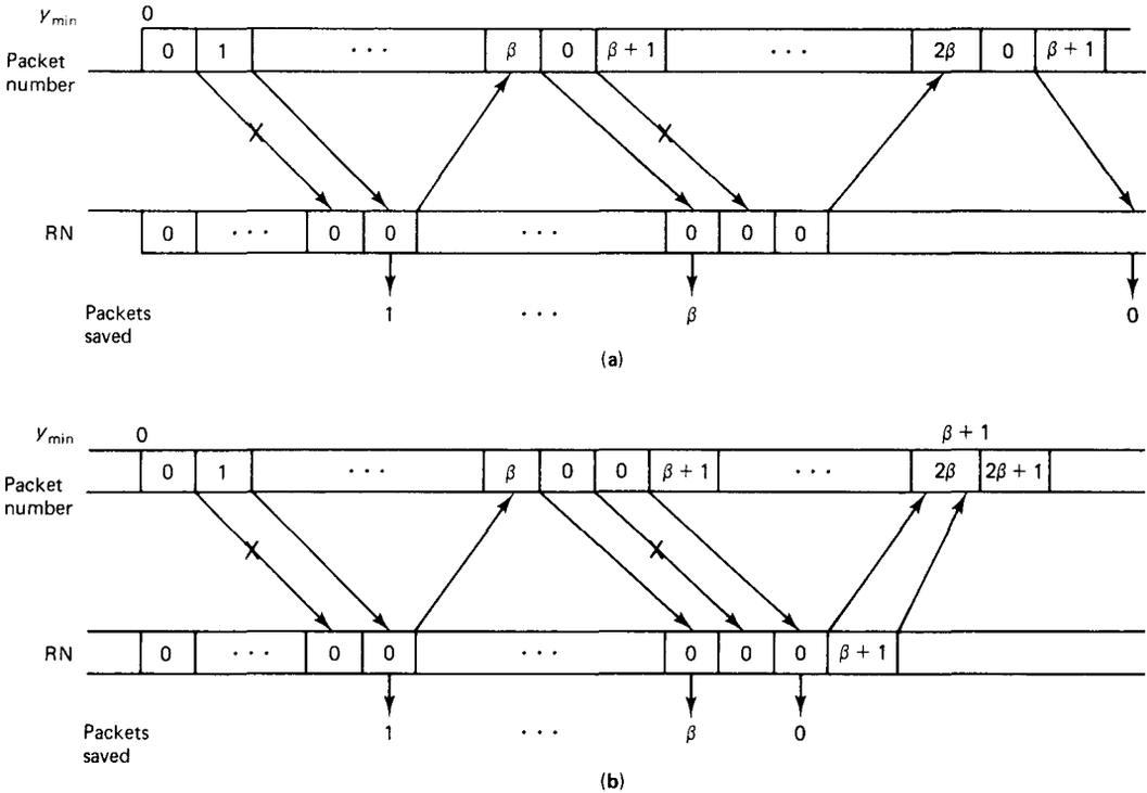
**Figure 2.32** Selective repeat ARQ with  $n = 2\beta + 2$  and receiver storage for  $\beta + 1$  packets. (a) Note the wasted transmissions if a given packet (0) is transmitted twice with errors. (b) Note that this problem is cured, at the cost of one extra frame, if the second transmission of packet 0 is doubled. Feedback contains not only  $R.N$  but additional information on accepted packets.
