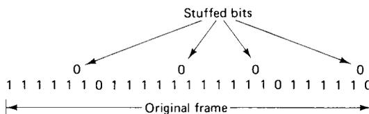
**Figure 2.36** Bit stuffing. A 0 is stuffed after each consecutive five 1's in the original frame. A flag, 0111110, without stuffing, is sent at the end of the frame.
