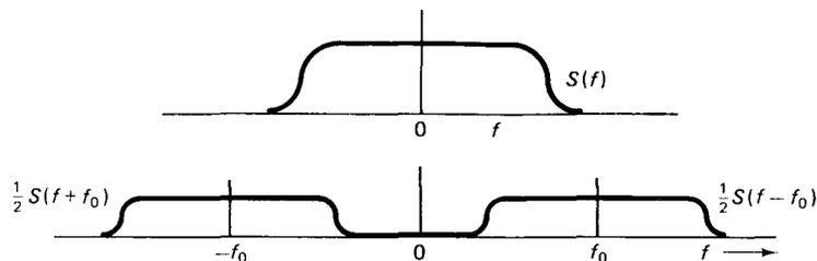
**Figure 2.10** Amplitude modulation. The frequency characteristic of the waveform  $s(t)$  is shifted up and down by  $f_0$  in frequency.
