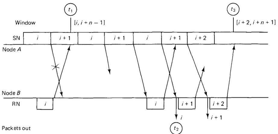
**Figure 2.28**  $SN_{min}$  is *i* at time  $t_1$ . Packet *i* is then released to the higher layer at *B* at time  $t_2$  and the window is increased at *A* at time  $t_3$ .
