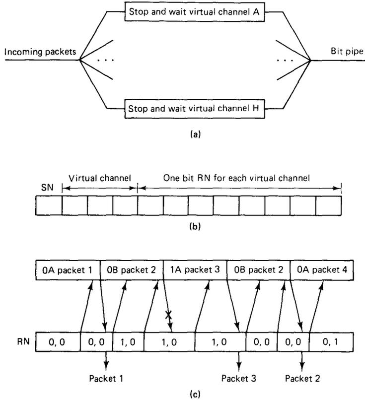
**Figure 2.33** ARPANET ARQ. (a) Eight multiplexed, stop-and-wait virtual channels. (b) Bits in the header for ARQ control. (c) Operation of multiplexed stop and wait for two virtual channels. Top-to-bottom frames show SN and the channel number, and bottom-to-top frames show RN for both channels. The third frame from bottom to top acks packet 1 on the A channel.
