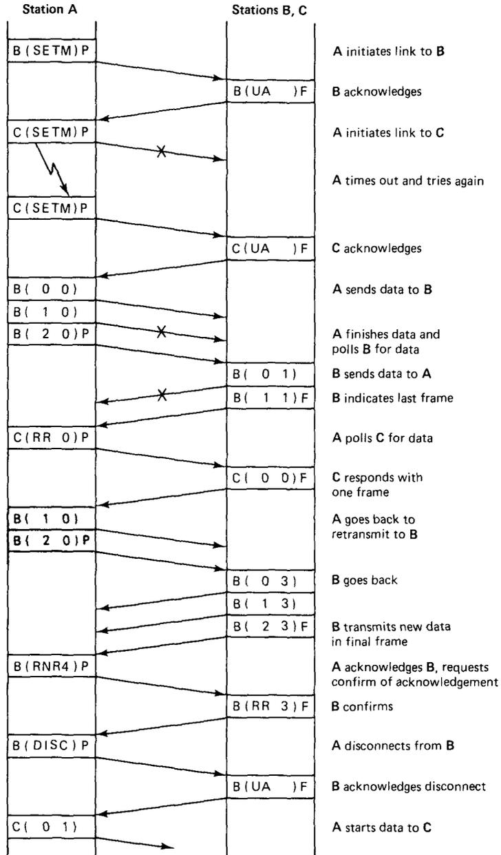
**Figure 2.40** Normal response mode (NRM) operation of primary A with two secondaries, B and C. SETM refers to the command setting, the NRM mode with SN = 0 and RN = 0 at both stations. The address of each frame is given first, followed by (SN,RN) for information frames, (type,RN) for supervisory frames, and (type) for unnumbered frames; this is followed by a P/F bit if set to 1. Note that A uses different SN and RN values for B and C.
