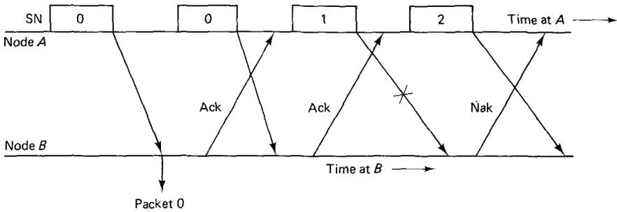
**Figure 2.19** The trouble with unnumbered acks. If the transmitter at *A* times-out and sends packet 0 twice, node *B* can use the sequence numbers to recognize that packet 0 is being repeated. It must send an ack for both copies, however, and (since acks can be lost) the transmitter cannot tell whether the second ack is for packet 0 or 1.
