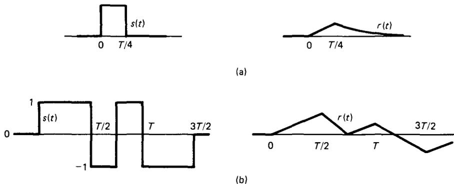
**Figure 2.4** Relation of input and output waveforms for the same channel as in Fig. 2.3. Here the binary digits enter at 4 times the rate of Fig. 2.3, and the rectangular pulses last one-fourth as long. Note that the output  $r(t)$  is more distorted and more attenuated than that in Fig. 2.3.
