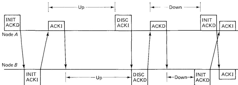
**Figure 2.45** Example of balanced initialization and disconnect protocol. Either node can start to initialize from the down state or start to disconnect from the up state and the other node will follow.
