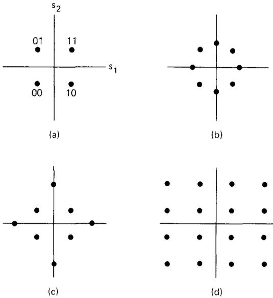
**Figure 2.12** Signal constellations for QAM. Part (a) maps two binary digits into a quadrature amplitude sample. Parts (b) and (c) each map three binary digits, and part (d) maps four binary digits. Parts (a) and (b) also can be regarded as phase-shift keying.
