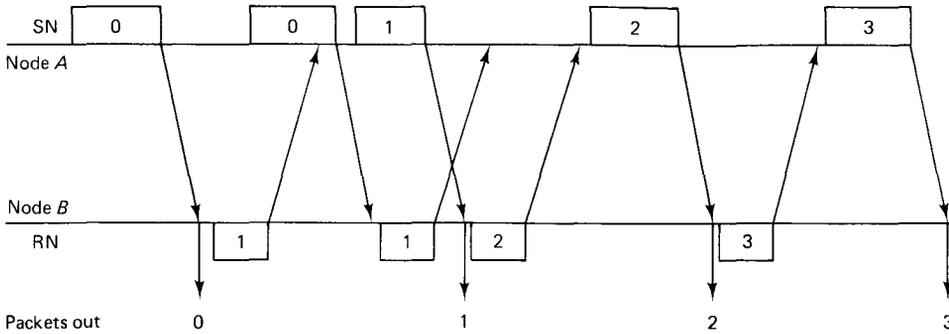
**Figure 2.21** Example of use of sequence and request numbers for stop-and-wait transmission from *A* to *B*. Note that packet 0 gets repeated, presumably because node *A* times-out too soon. Note also that node *A* delays repeating packet 1 on the second request for it. This has no effect on the correctness of the protocol, but avoids unnecessary retransmissions.
