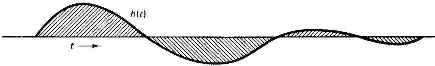
**Figure 2.8** Impulse response  $h(t)$  for which  $H(f) = 0$  for  $f = 0$ . Note that the area over which  $h(t)$  is positive is equal to that over which it is negative.
