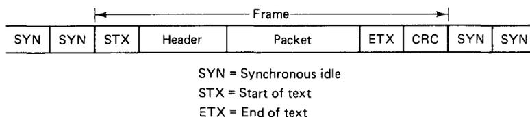
Figure 2.34 Simplified frame structure with character-based framing.
