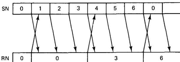
**Figure 2.31** Go back 7 ARQ with long frames in the reverse direction. Note that the ack for packet 1 has not arrived at the sending side by the time packet 6 finishes transmission, thereby causing a retransmission of packet 0.
