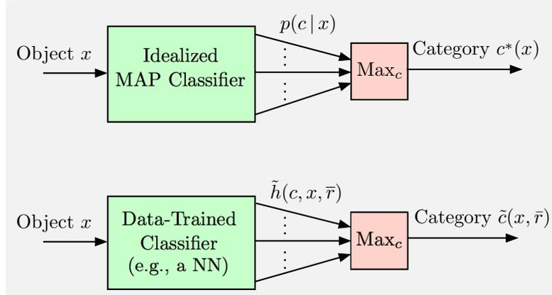
**Figure 3.5.1.** Illustration of the MAP classifier  $c^*(x)$  for the case where the probabilities  $p(c|x)$  are known [cf. Eq. (3.37)], and its data-trained version  $\tilde{c}(x, \bar{r})$  [cf. Eq. (3.41)]. The classifier may be obtained by using the data set  $(x_k^s, u_k^s)$ ,  $s = 1, \dots, q$ , and an approximation architecture such as a feature-based architecture or a neural network.
