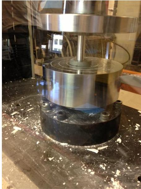
*Fig.2.4* Aluminum sample between the compression anvils.
