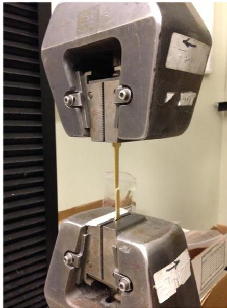
*Fig. 2.2* Brass sample between the lower base and upper fixture that had undergone uniaxial tensile testing.
