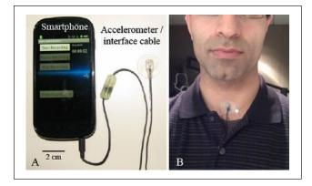
**Figure 1.** Illustration of the accelerometer-based ambulatory voice monitor. (A) Smartphone, accelerometer sensor, and interface cable with circuit encased in epoxy and (B) wired accelerometer mounted on a silicone pad affixed to the anterior neck surface midway between the thyroid prominence and the suprasternal notch.
