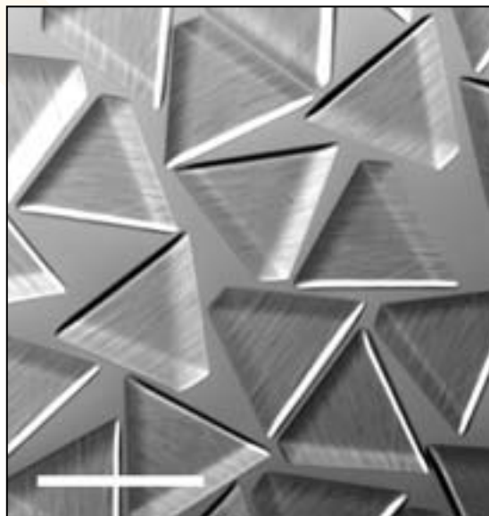
CFL allows nonspherical particles to be fabricated quickly and easily. Scale bar = 100 \mu\text{m} .
