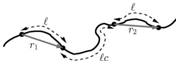
FIG. 1. Illustration of a worm-like chain with vectors connecting positions on the chain. The coarse-grained model would ideally reproduce the average correlation of the vectors. The polymer has persistence length A_p . The contour length represented by the vectors is \ell . The contour length between the two vectors is \ell_c .
