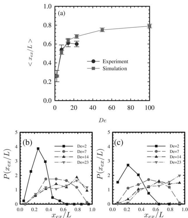
**Fig. 3** (a) Comparison of mean fractional stretching ( $\langle x_{ex}/L \rangle$ ) obtained in experiments<sup>10</sup> and simulations. DNA stretching ( $x_{ex}$ ) is measured when the downstream-most part of a DNA passes the exit of the funnel ( $x/l_c = -1$ ). Probability distribution of mean fractional stretching: (b) experimental results and (c) simulation predictions.
