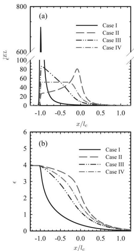
**Fig. 4** Non-dimensionalized strain rate (a), and strain (b) for four funnel shapes along the channel centerline ( $y = 0$ ). The detailed information for the funnels is provided in Table 1.
