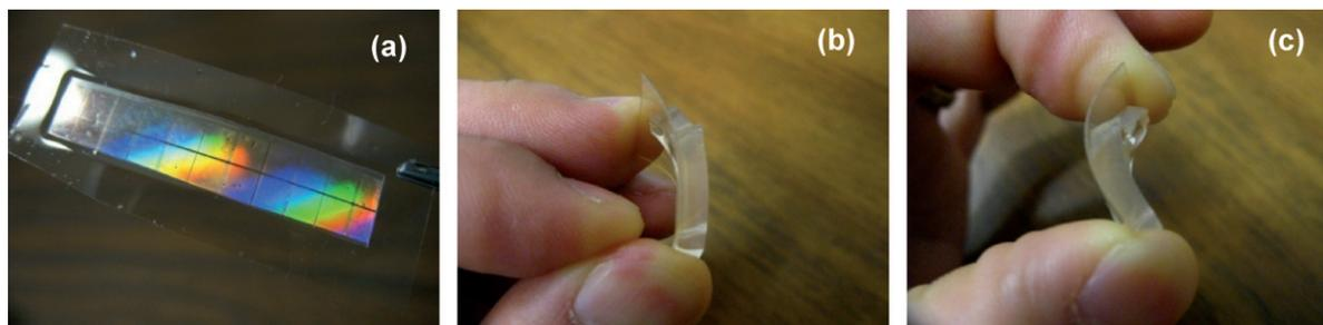
**Fig. 2** Pre-patterned PU substrate bonded with PC film (a) and compressive (b) and tensile (c) stresses were applied to a test microfluidic device composed of pre-patterned PDMS substrate bonded with PET film.
