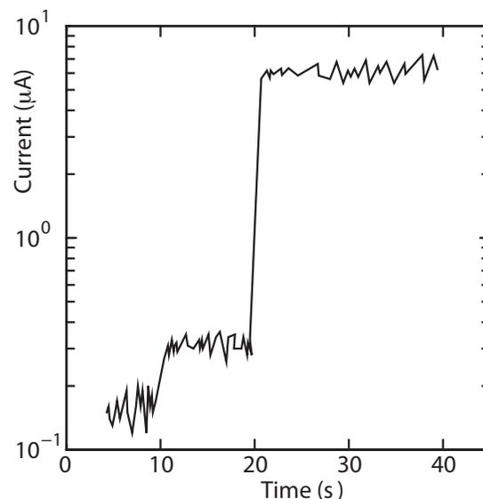
**Fig. 2** Current through the array of  $200 \times 250 \text{ nm}^2$  channels with an applied voltage of 200 V across the loading reservoirs. Initially, the channels contain  $1 \times \text{T}$  buffer. At times  $t = 10$  and 20 s, solutions of 30 mM and 2 M NaCl, respectively, are exchanged through the perpendicular, intersecting array of  $200 \times 150 \text{ nm}^2$  channels into the  $200 \times 250 \text{ nm}^2$  channels.
