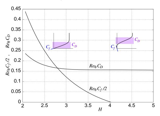
Laminar  $C_{\mathcal{D}}$  is very insensitive to pressure gradient — dissipation region just moves on/off the surface
