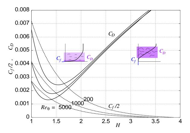
Increased mixing increases  $C_{\mathcal{D}}$  in adverse pressure gradients Note: A turbulent free shear layer has  $C_{\mathcal{D}} \simeq 0.02$  (!)
