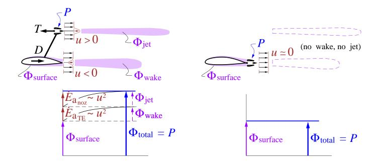
Isolated propulsor:  $P = \Phi_{\text{total}} = \Phi_{\text{surface}} + \dot{E}_{\text{a}_{\text{TE}}} + \dot{E}_{\text{a}_{\text{noz}}}$
