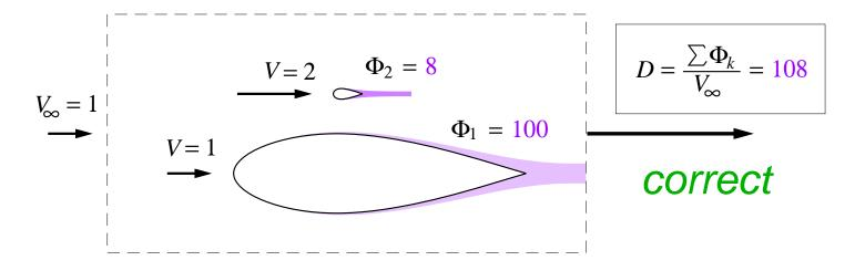
Dissipation Build-Up captures "mystery interference drag", which cannot be estimated via simple Drag Build-Up.
