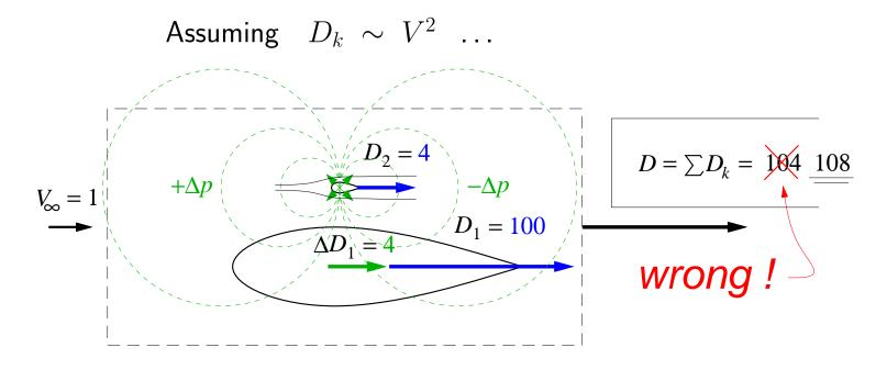
Also present is buoyancy drag  $\Delta D_1$  on large body, due to small body's source-disturbance pressure field  $\Delta p$ .
