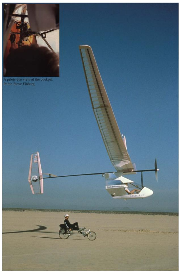
Ryan recumbent cycle paces Daedalus 'A' over the vast flats of Edwards air force base in California. Significantly, with experienced cyclists the aerodynamic efficiency of the human powered aircraft enables airscrew drive to match the effort required for the wheeled bicycle. Photo Steve Finberg
