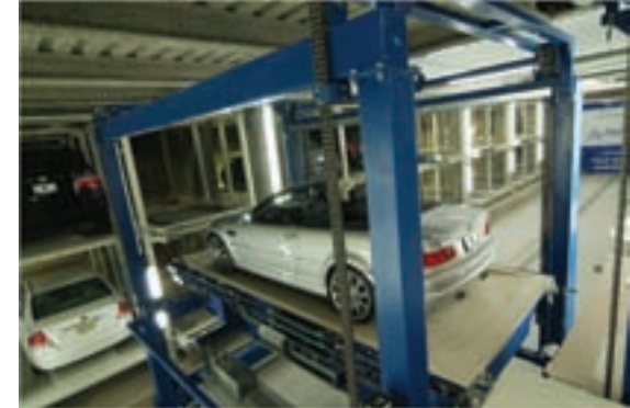
Automated Parking Garage by Stolzer Parkhaus > This high-efficiency garage allows for increased security, simplicity, and efficiency for both the parking customer and developer, despite the fact that the structure is underground. A customer can retrieve his car within three minutes. Source: New York Times.
