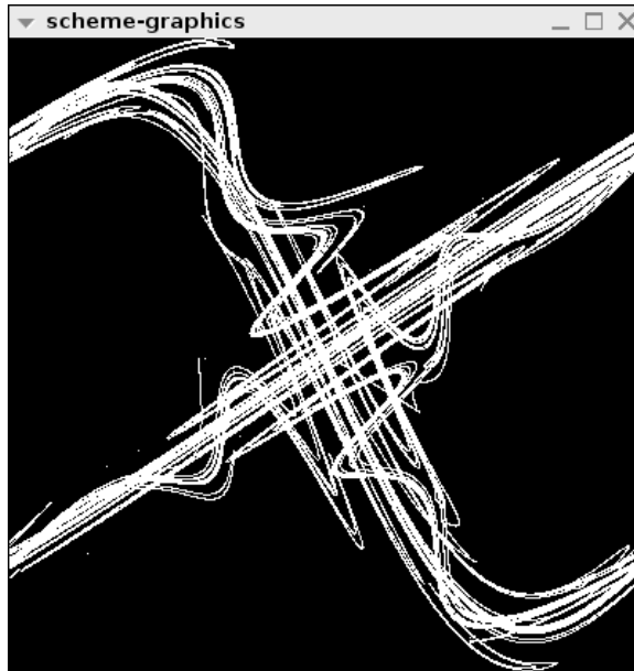
Figure 2: Computed stable and unstable manifolds around the (I = 0, \theta = 0) fixed point of the K = 1.5 standard map. The axes are -\pi \leq \theta \leq \pi and -\pi \leq I \leq \pi .
