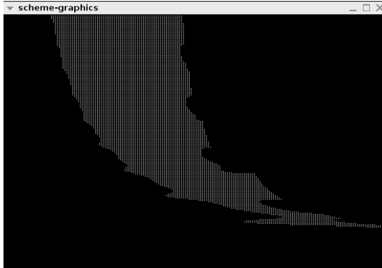
Figure 2: Region of parameter space for which an inverted equilibrium exists. The ordinate is 0 \leq \omega \leq 10 . The abscissa is 0 \leq A \leq 10 . The points are spaced \Delta A = \Delta \omega = .05 apart.
