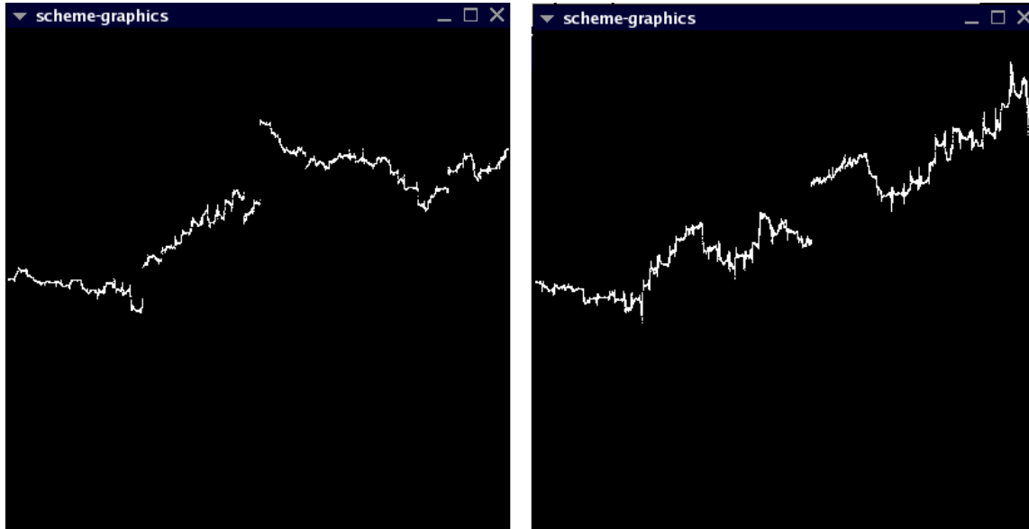
Figure 3: Total energy of the double-pendulum system from t = 0 to t = 50 , with step size of \Delta t = .005 . The y-axis goes from -10^{-10} to 10^{-10} .
