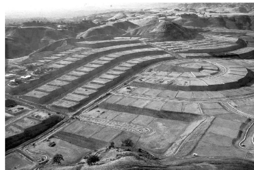
Fig. 2. Attempts to reshape development are often thwarted by engineering standards and procedures. Impacts can be seen in the administration of street layouts and widths as well as grading and drainage practices. One of the most troublesome stages in the site development process involves the clearing of vegetative cover and mechanical standardize grading. Source: Courtesy of Alex MacLean, Landslides.
