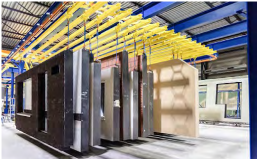
▲ Energiesprong pre-fabricated insulation walls for quick installation ▶
