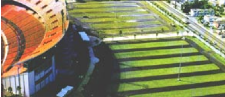
figure 2: surface parking of a stadium covered with grass, allowing higher permeability for storm water.
