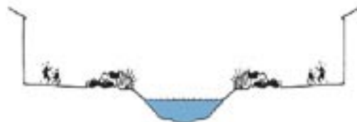
figure 8: Natural canal integrated with streets, section 图 8：自然水道与街道整合，截面
