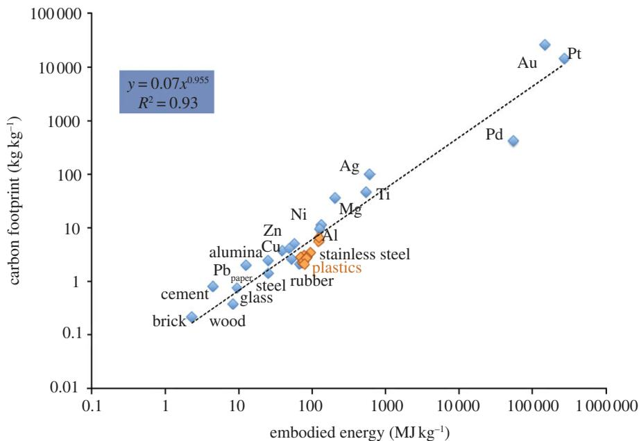
**Figure 2.** The carbon emission in kilograms of CO<sub>2</sub> per kilogram of material produced versus the embodied primary energy. Data adapted from Ashby [10].
