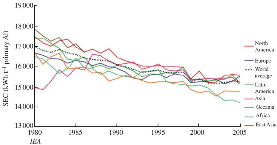
**Figure 5.** Historical regional data for the energy (electricity) intensity of aluminium smelting. SEC, specific energy consumption. Reproduced with permission from IEA [7]. Tracking industrial energy efficiency and CO<sub>2</sub> emissions © OECD/IEA 2007, figure 8.1, page 211.
