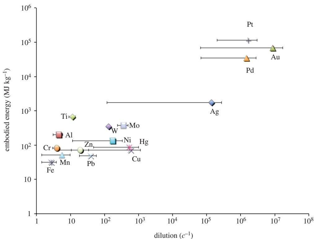
**Figure 3.** Embodied primary energy of 16 metals [10] plotted against the dilution, or inverse of concentration, of the common ores used to produce the metals [12].
