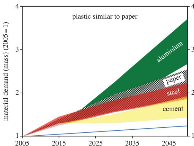
**Figure 8.** The range of future demand for aluminium, paper, steel, plastic and cement constructed from forecasts provided by the IEA [7]. Plastics demand projection adapted from Allwood *et al.* [5]. The bottom curve (blue) leading to 1.25 in 2050 shows the maximum demand allowed in order to meet the goal of halving the world's energy use by materials with a 56% improvement in energy intensity (see text).
