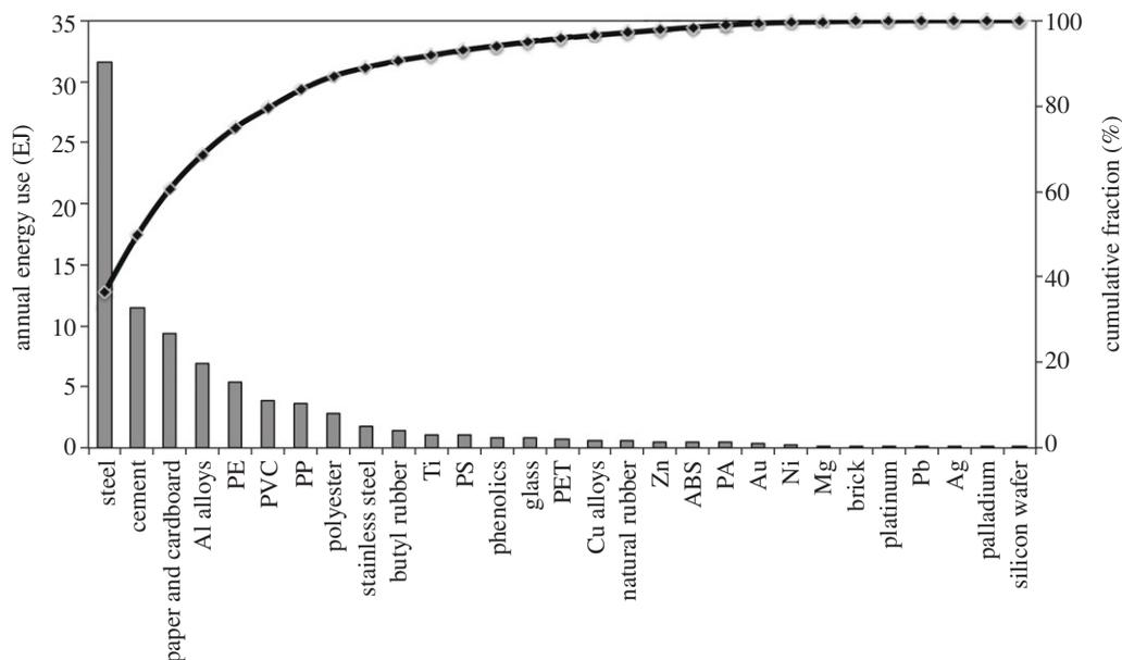
**Figure 1.** Annual primary energy used for the production of 29 materials worldwide, cumulative scale on the right. PE, polyethylene; PVC, polyvinyl chloride; PP, polypropylene; PS, polystyrene; PET, polyethylene terephthalate; ABS, acrylonitrile butadiene styrene; PA, polyamides. Adapted from Ashby [10].
