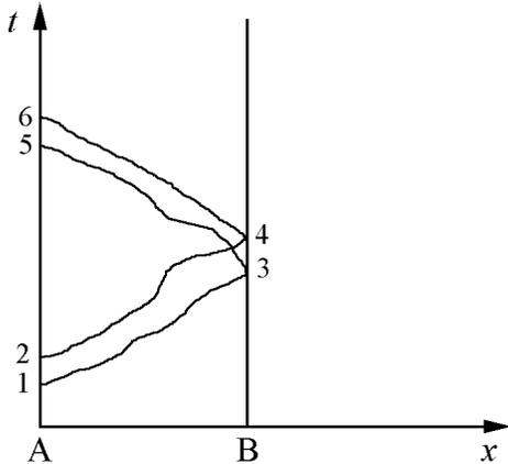
Figure 1: Setting up a coordinate system in curved spacetime. There are two time-like worldlines and two pairs of null geodesics. The appearance of flat coordinates is misleading; the metric varies from place to place.
