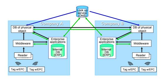
With this structure, identification of individual units becomes possible though the electronic product code (EPC), which has the capability for unique identification of trillions of items. Unique identification on this scale results in useful information for track and trace (Koh et al. 2003a; Schuster and Koh 2004), the authentication of objects located anywhere in a supply chain (Koh et al. 2003b), and the management of versions of the same item code (Engels et al. 2004).
