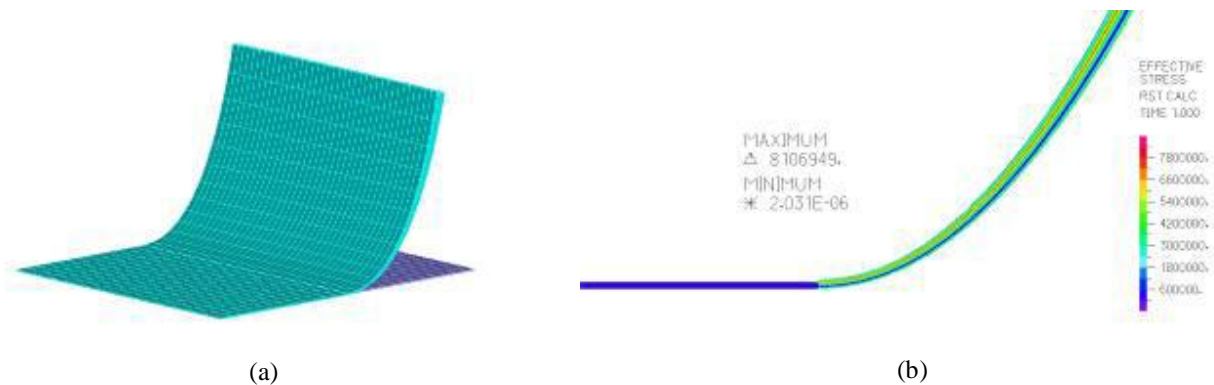
Figure 3: (a) FEM showing the post-release behavior of a stressed metal bilayer hinge; (b) Stress profile through the thickness of the hinge.
