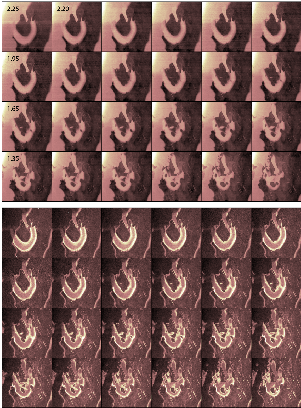
Figure C-5: 10 \times 10 \mu\text{m} \nu = 2 hole bubble tip bias voltage sweep from -2.25 to -1.00 V at 2.6T. A “donut” charge perturbation is visible in the images.
