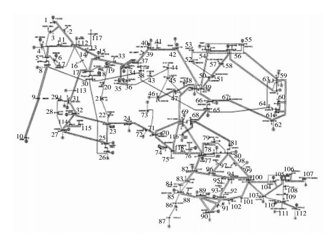
Fig. 6. One line diagram of 118 bus (power flow test case) system
