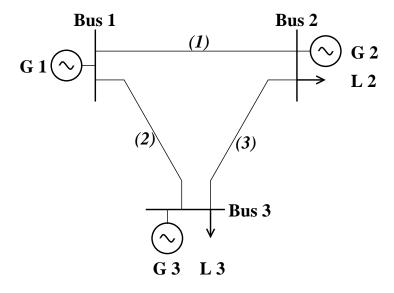
Fig. 3. One-line diagram of 3-bus electric power network
