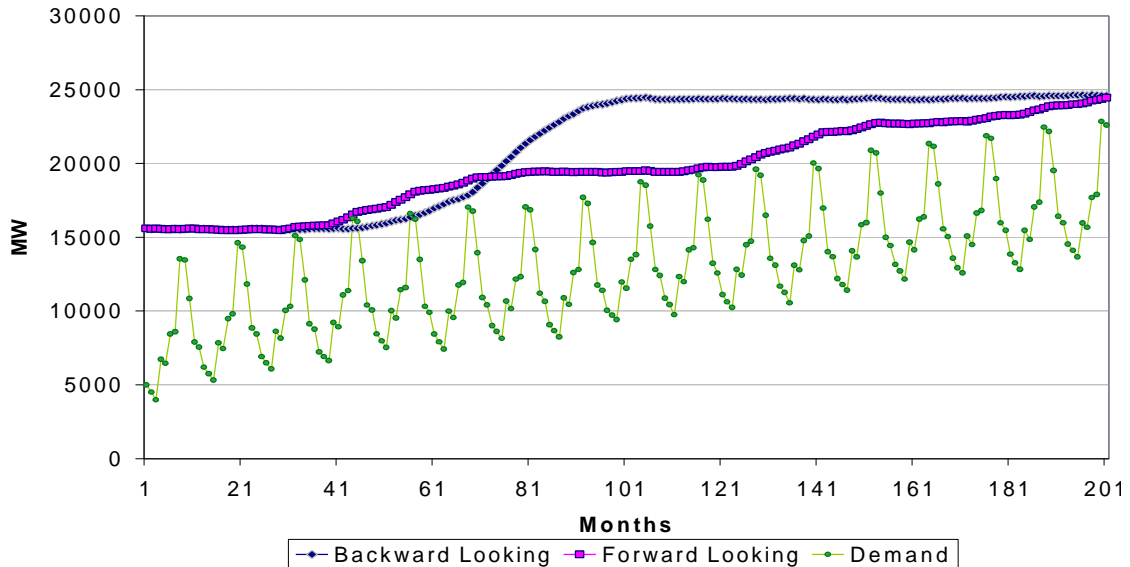
Figure 4.12 Supply Capacity and Demand: with Seasonal Demand and 24-period Time Delay \tau \geq P
