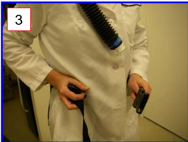
Fasten belt around your waist with motor/battery assembly at your lower back. It helps to put supply air tube over your shoulder.
