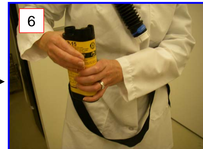
Clip the battery onto the side of the belt.
