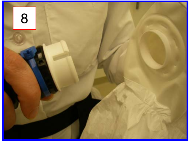
Connect supply air hose to fitting at the back of the Tyvek hood. Make sure it is tight and cannot be easily tugged out.
