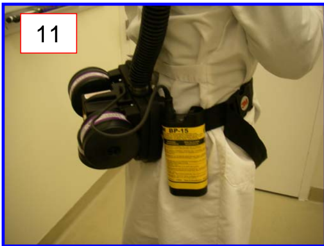
The final motor/battery/belt assembly should look something like this
