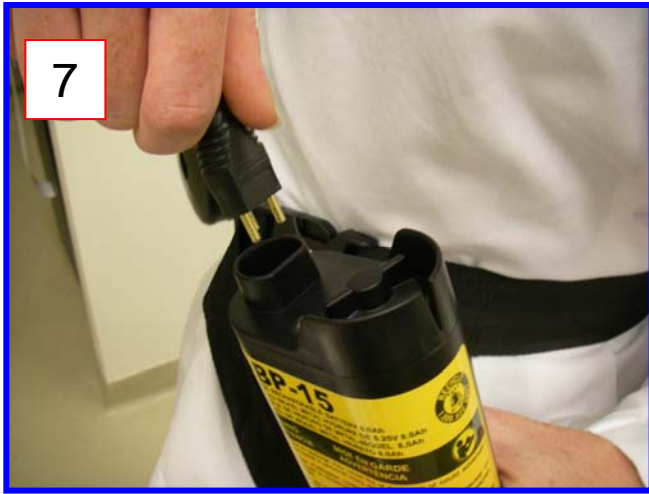
Plug the motor into the battery.
