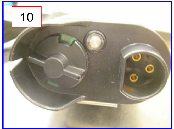
Turn the switch on the battery to the "ON" position (green)
