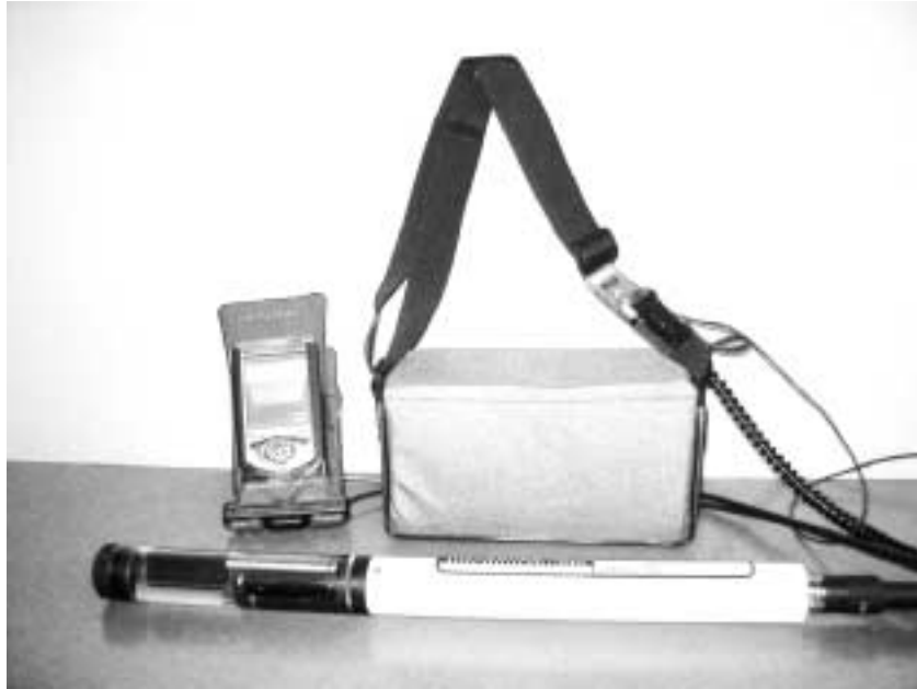
Figure 2: Hardware components for the prototype ENVIT Field Notebook Data Collection System.
