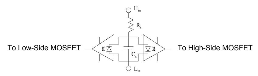
$V_{sig}$ =3.3V,  $R_s$ =200 $\Omega$ ,  $C_s$ =0.047 $\mu$ F, Synchronous Rectification 8.5 $\mu$ s (using the equation for the previous slide) Conditions:
