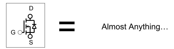
Because the floating supply and optocoupled gate driver are very modular, the MOSFETs used can be virtually anything. They can be individual small MOSFETs, many small MOSFETs in parallel, or large MOSFETs with huge current-handling capabilities. They can be in almost any configuration, including half- and full-bridges. The modular gate driver treats high- and low-side MOSFETs the same. There are a few general guidelines to follow:
