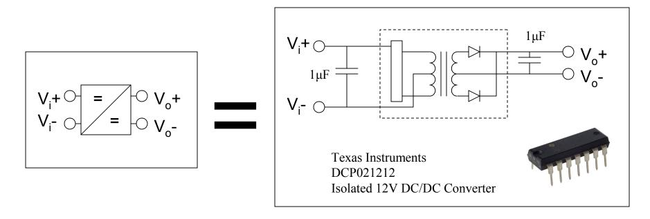
The **Texas Instruments DCP021212** is an isolated 12V to 12V DC-DC converter. It takes a 12V input, referenced to a common ground, and outputs 12V referenced to some other voltage. It uses AC and magnetic coupling to isolate the output from the input. This is used to supply +12V referenced to a MOSFET source pin, no matter where that is with respect to the system ground.
