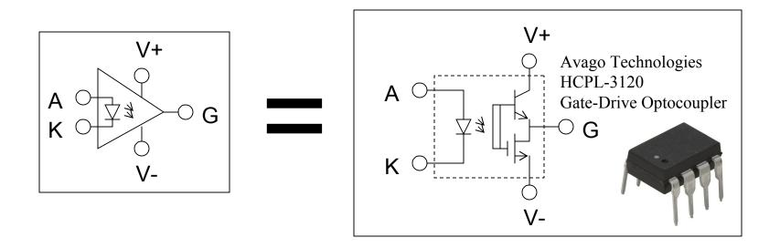
The **Avago HCPL-3120** is an optically-coupled MOSFET or IGBT gate driver. The purpose of optical coupling is to isolate the input signal from the high-power electronics. When the LED is on, the MOSFET gate is sourced by V+. When the LED is off, the gate is sunk to V-.
