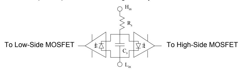
The above circuit is a passive way to ensure that shoot-through cannot occur in a half-bridge. It introduces a delay between turn-off of one MOSFET and turn-on of the other. Note that the optocoupler LEDs are in reverse-parallel configuration.
