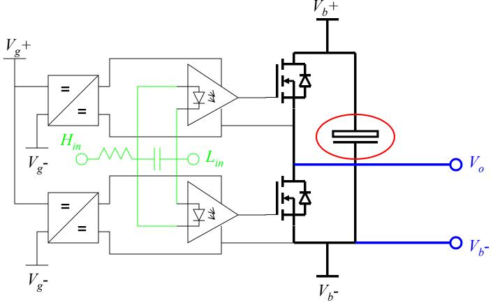
The input capacitance holds the voltage across the half-bridge stable against inductive voltage spikes from the battery cables. Its exact value depends on many factors, but a very conservative worst-case estimate can be made by consindering the voltage ripple if the battery cable inductance was very large:
