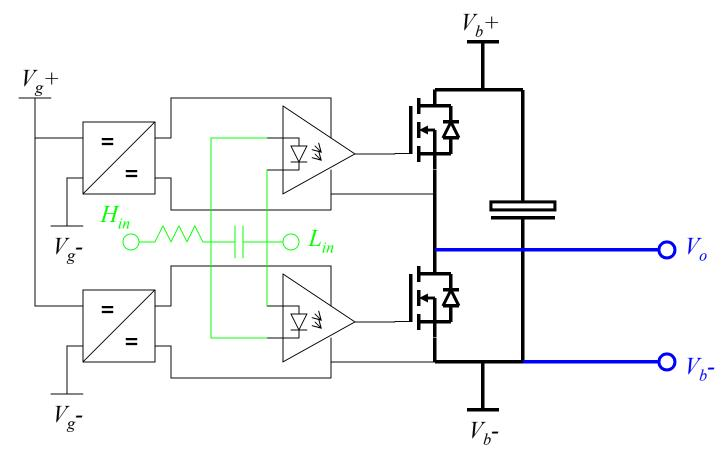
$V_g$ - (gate drive supply ground),  $V_b$ - (main power supply ground), and logic ground for optocoupler inputs are all isolated! You can do whatever you want with them. If everything is supplied by one battery, all grounds will be the same. You can tie grounds together with small resistors and use lots of extra capacitance to protect the logic from noise on the power ground. Or, you can supply the logic and/or gate drivers with a separate battery for complete isolation.
