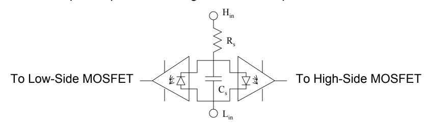
$R_s$  should be chosen like a standard LED current-limiting resistor:
