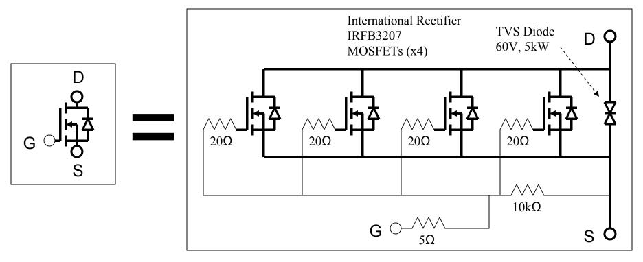
**IRFB3207:** These are serious workhorse MOSFETs. Even though they are in a small TO-220 package, each one can handle 75A at 48V if properly heatsinked.
