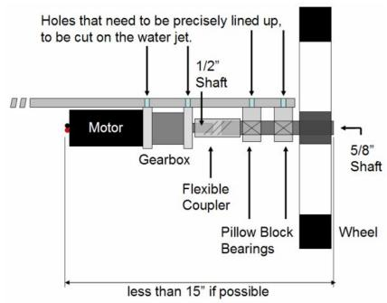
Quick PowerPoint sketch of the proposed direct-drive assembly. The bearings support the full weight of the segway and rider so that the gearbox shaft has very little sideways force on it. We will need to do a SolidWorks model of this next meeting.
