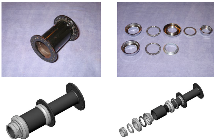
Hub design, before and after, clockwise from top left: Current hub produced in TZ, common bicycle stem bearings, exploded view of bearings used on new hub design, assembled new hub design
