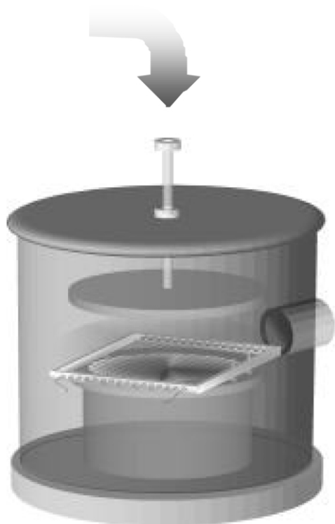
Fig. 1. Schematic of the HWCVD chamber. Showing gas inlet through upper showerhead, pyrolysis on square filament array, and deposition onto a wafer substrate resting on the bottom electrode. The gas pump out is toward the back side of the chamber.
