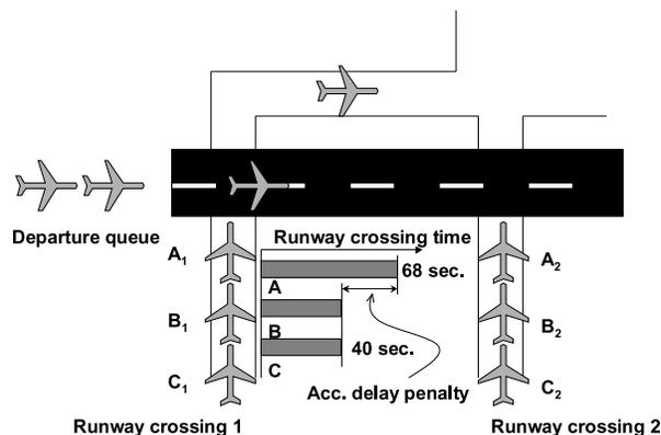
Figure 4: Schematic of a departure runway with two active runway crossing queues.
