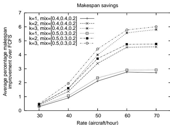
Figure 2: Average throughput improvement over FCFS for basic departure scheduling with 10-min departure time-windows.
