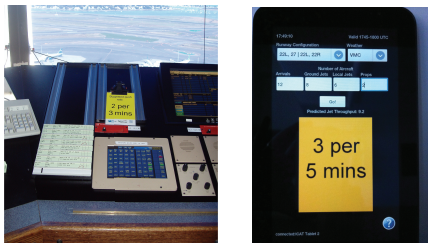
Figure 3: (Left) Display of a pushback rate control card in the Boston airport tower; (right) Tablet-based rate control input interface [40].
