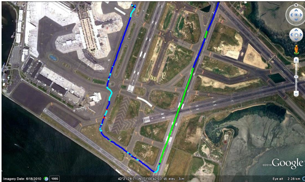
(b) Departing flight: Departure is on Runway 4R, with acceleration phase indicated in green.
