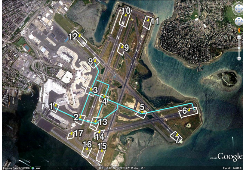
Figure 1. Network model of Boston (BOS) airport. Nodes are marked using white boxes. The links highlighted in light blue constitute the configuration-specific network for departures from Runway 27.
