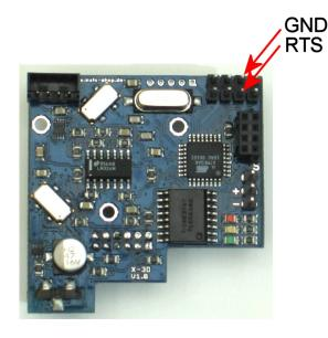
Alternatively, you can use the pin as an input for a radio modem's RTS (Request To Send) pin. The X-3D-BL Scientific will only send data if the RTS pin is pulled low by the connected device. It will stop sending data if the Pin is pulled high by the modem to prevent data loss during the transmission.
