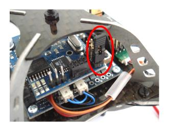
Connect the USB-adapter to your computer. Open the X-Control software, click on "X-3D" and on the left hand side on "X3D firmware upgrade". Then, connect the X-3D to the USB adapter as seen in the following picture.
