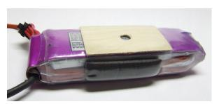
The black foam on both sides hinders it from being hurt by the magnesium parts of the frame. The woodden plate on the bottom makes it stick to the screw holding the bottom plate of the frame. Of course, there are many different ways to prepare your battery for a safe operation. This is only an example.
