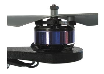
Please note that there are two types of propellers: One pair of propellers is spinning clockwise, the other pair is spinning counterclockwise. The propellers spinning clockwise must be mounted to the front and the rear motor, whereas the counterclockwise rotating propellers must be mounted to the left and to the right motor.
