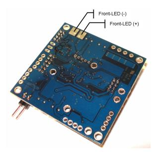
An LED connected to the "Front-LED" Pads on the bottom side of the X-Base will always be on as long as the X-3D-BL is turned on. Such an LED can be mounted to the very front of your vehicle to make it easier for the pilot to know where the front side is.
