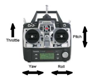
The X-3D-BL scientific works with any R/C with at least five channels. Make sure that all channels work independently and that no mixers are active in your remote.
