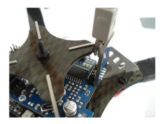
Open the X-Control software and click on "X-Base". Choose the correct COM-Port (normally "Autoselect: COMxx") and click on "Connect". Chose "X-BL Setup" and click on "start search". After several seconds four brushless controllers with different serial numbers should appear in the list. If less than four controllers appear, turn of your X-3D-BL, check all solderings and connectors and repeat the previous steps.
