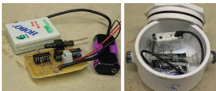
Figure 3. Pictures of circuit (left) and waterproof housing with packaged electronics (right).
