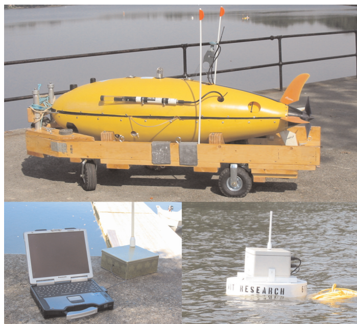
Fig. 1. Components of the NEREUS network include an Odyssey II AUV equipped with mass spectrometer and water quality microprobe (top), several buoys that contain fixed sensors and serve as wireless and acoustic communication nodes (bottom right), and a shore station that logs data, provides real-time displays, and issues commands (bottom left).
