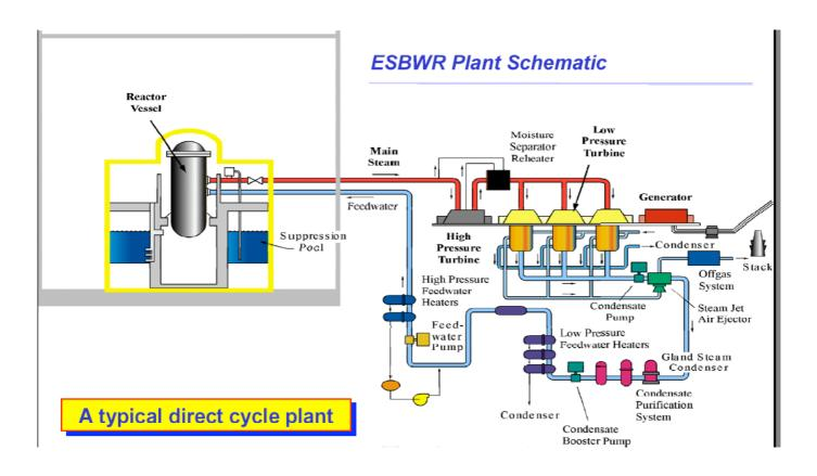
Figure 2 and 3: SBWR Plant and Containment Systems Schematic Diagrams
