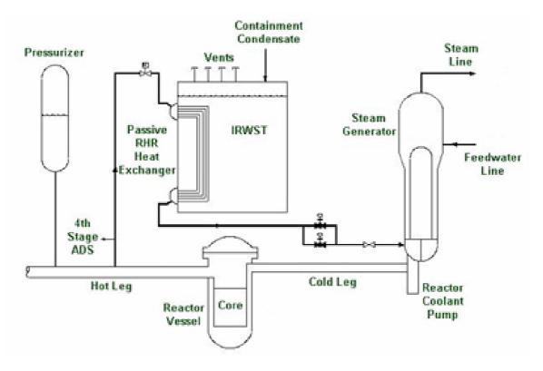
Figure 5: Passive Safety Features of the AP600 and AP1000 Reactor Designs
