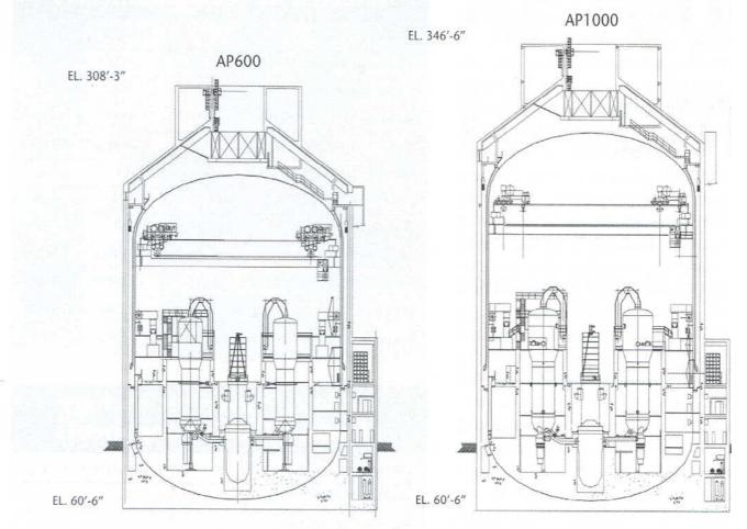
Figure 4: AP600 & AP1000 Comparison and Overall Plant Conceptual Figure
