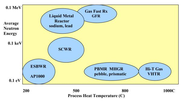
Figure 1: Conceptual Mapping of Generation IV Nuclear Reactor Concepts
