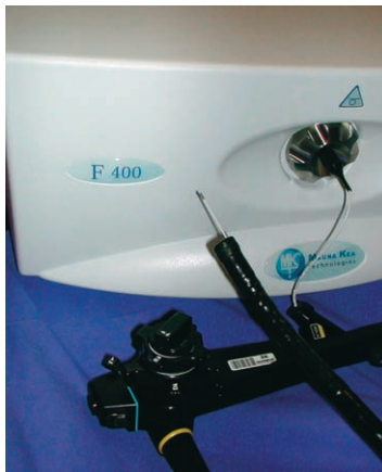
Fig. 22. Prototype in vivo confocal microendoscopy system from Mauna Key Technologies, France. The system comprises a central unit, dedicated image processing and analysis software, and a handheld endoscopic probe (see insert). (Courtesy of Mauna Kea Technologies, Paris, France.)
