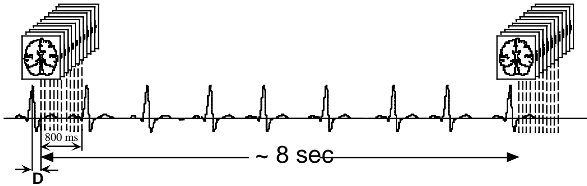
Figure 4: Timing of image acquisitions relative to the subject's EKG for the functional image data in directory Lab3.2a.
