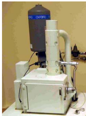
Fig. 21 Portable SEM at Ecole Polytechnique in France to be used in conjunction with a tensile loading frame for in-situ testing.
